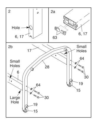
3. Raise the Uprights (6, 17) to the vertical position. Place the Frame (55) between the Uprights as shown.
